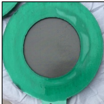
Figure 7. Compressor outboard bearing approved first pass inspection screen 2/23/18
