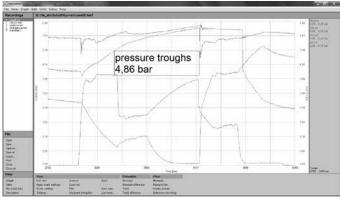
Overlay of curves, for example to document the wear of a machine (new condition/current condition)
