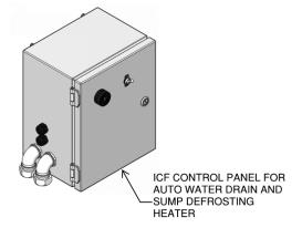
Note: Filter Sump Heater Control Panel dimension: 6.5" W x 5.5" H x 6.5" D (165 W x 140 H x 165 D) Automatic Water Drain Control Panel dimension:10" W x 8" H x 12" D (254 W x 203.20 H x 304.80 D) \*For use above 32°F (0°C) only Electrical cable length (Control Panel to ICF): 4 ft. (1.22m) Hose length for Automatic Water Drain feature (ICF to Tank): 6 ft.(1.83m) All control panels "NEMA 4X" rated  $\Delta \boldsymbol{\mathsf{P}}_{\mathsf{element}}$
