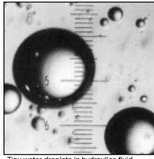
Tiny water droplets in hydraulics fluid (1 unit equals 10 micron)
