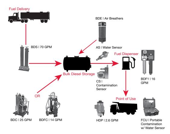
HYDAC has developed many of these core diesel products into turnkey filtration solutions with integrated pump motor functions for almost every diesel application from gen sets to fleet fueling tanks to the Ag tank at a farm. All are designed to address the challenges of fuel in its environment.
