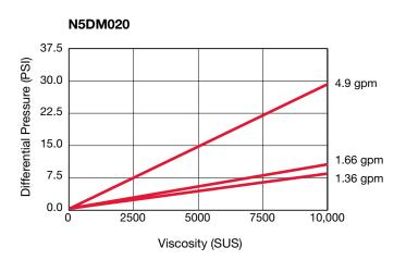
SRV Flow Control Valve Curve
