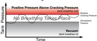
When fluid level rises, the existing air volume is compressed, and no air is expelled until the cracking pressure is surpassed.
