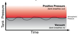
When fluid level rises, the tank pressure rises and air is immediately expelled through the breather whenever positive pressure exists.
