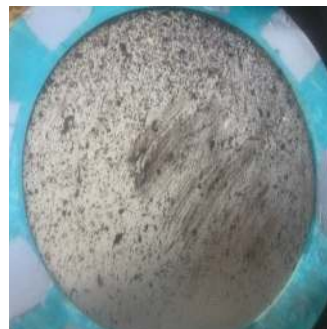
Before After API 614 Screen on 6" Return Line
