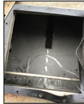
Figures 12a & 12b. Interior of the Wet Gas lube oil reservoir before cleaning (left) and post cleaning (right).
