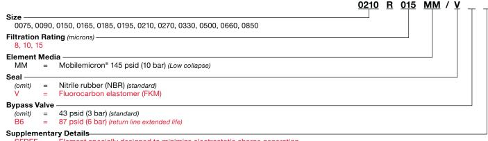
SFREE = Element specially designed to minimize electrostatic charge generation
