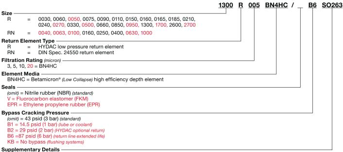
SO263 = Modification of ON & W/HC elements for Skydrol or HYJET phosphate ester fluids
