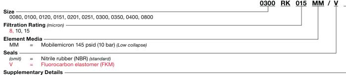
SFREE = Element specially designed to minimize electrostatic charge generation
