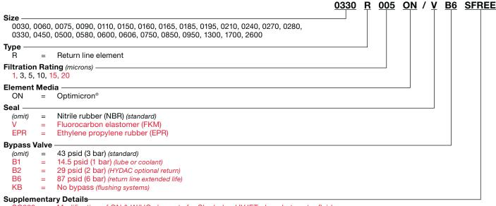
SO263 = Modification of ON & W/HC elements for Skydrol or HYJET phosphate ester fluids SFREE = Element specially designed to minimize electrostatic charge generation
